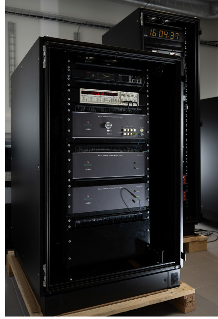
Figure 4: Photography of the 19'' integrated Rolex Rubidium Optical Atomic Clock prototype.
